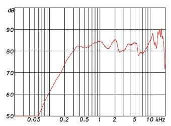
RL 110 AX max. SPL @ 3% and 10% distortion threshold 30 W max. Power
